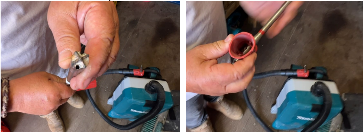
Close-up of the dust-extraction drill bit showing the vacuum holes in the bit
