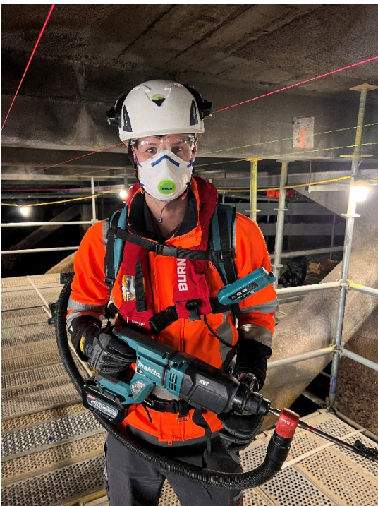
Worker wearing the backpack-mounted vacuum demonstrating ergonomics and mobility
