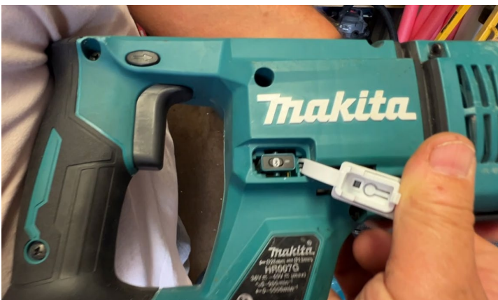
Detail shot of drill and vacuum setup highlighting Bluetooth-connected battery tools
